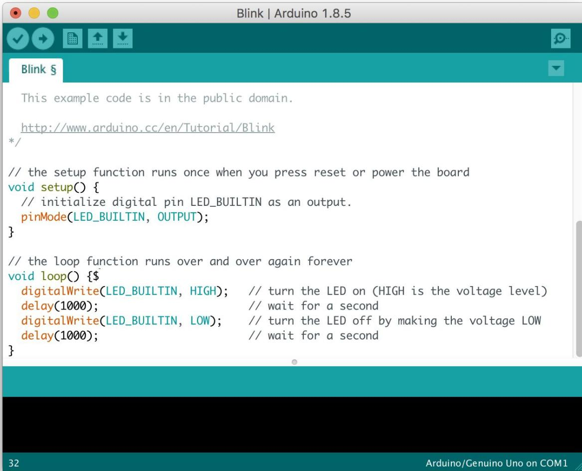
The screenshot shows the Arduino IDE interface with the title bar "Blink | Arduino 1.8.5". The main window displays the "Blink" example sketch. The code is as follows:
